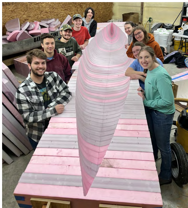
Concrete Canoe Foam Mold
