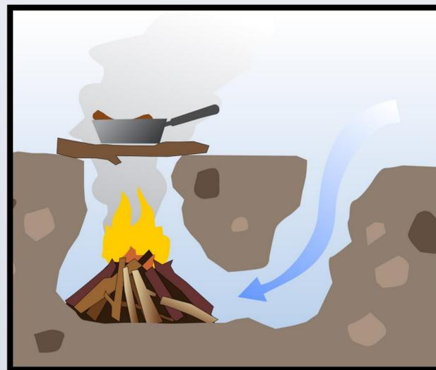
Figure 1: Illustration of a Dakota Fire Pit
