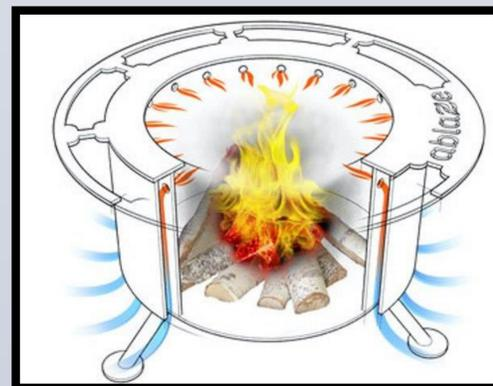
Figure 2: Inner-Workings of a Modern SCP
